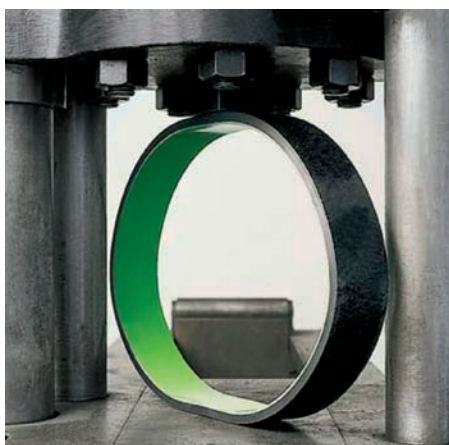
The PUR coating adheres exceptionally well to the cast-iron surface.
